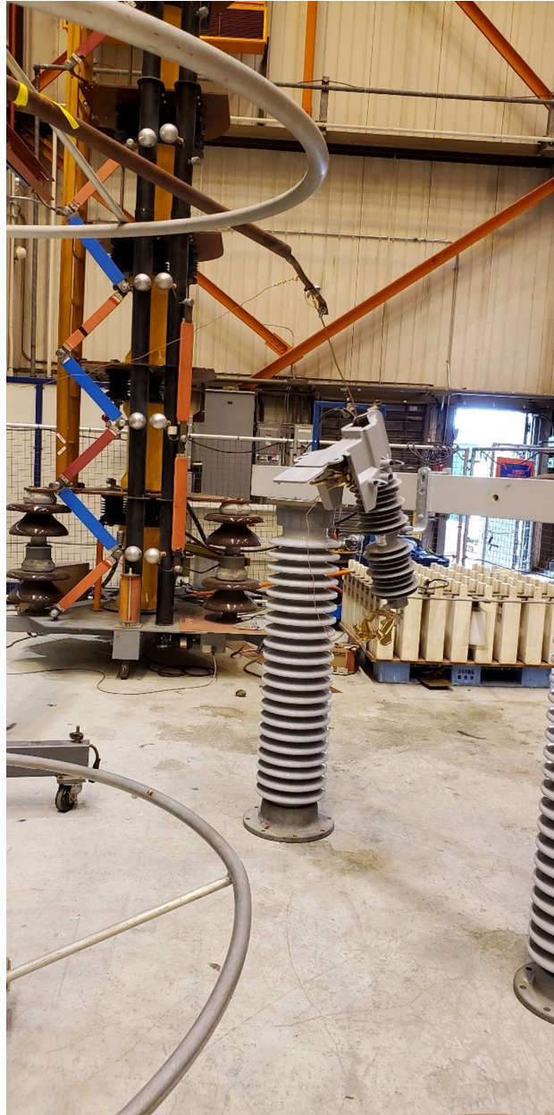
Figure 7. Lightning impulse withstand test setup
