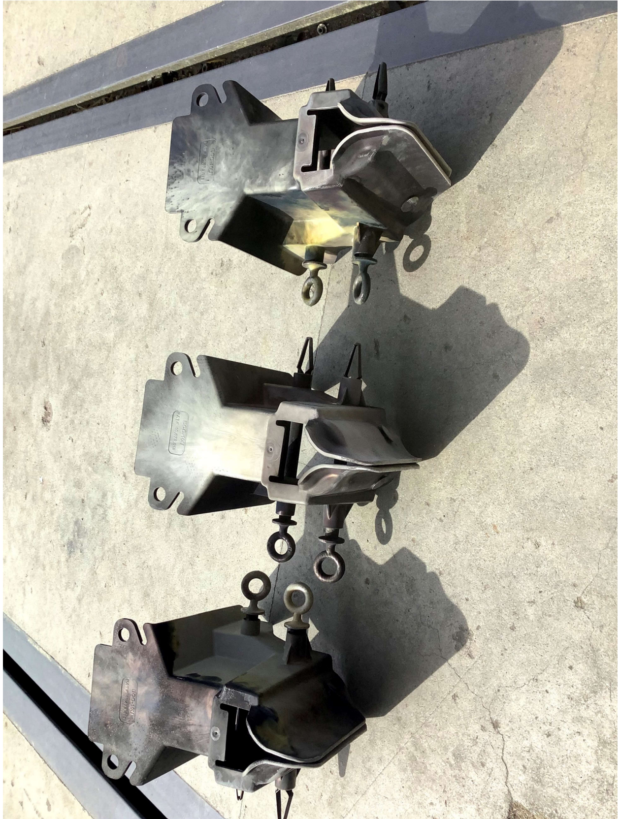
Figure 12. Samples after the high current (power arc) tests.
