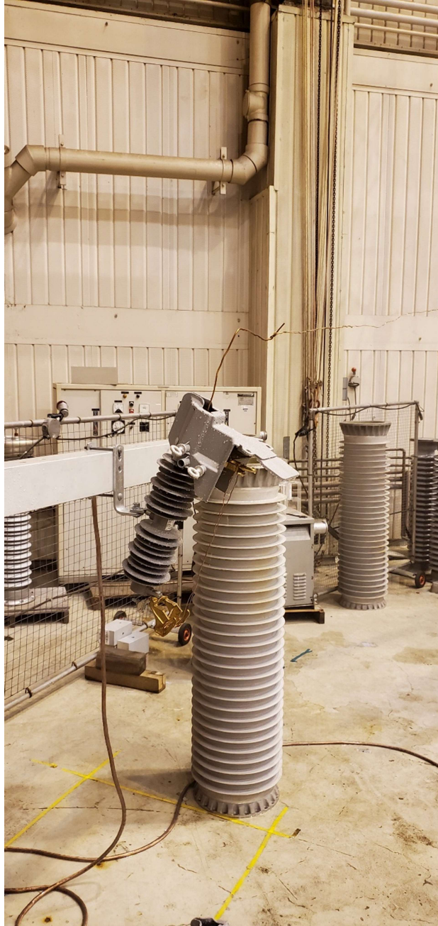
Figure 8. Wet withstand and wet power-frequency flashover test setup
